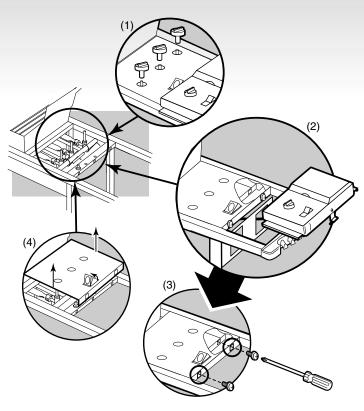
5) Replace control panel when Leak Check is completed.
